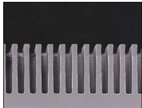
Etched Trenches 10 \mu\text{m} features, 65 \mu\text{m} deep (Photo Courtesy of ULVAC)
