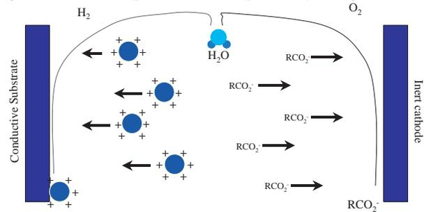
Figure 3. Electrodeposition of the positively-charged Micelle
